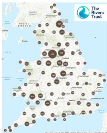
There are around 15,000 storm overflows in England. They discharge at different rates depending on local conditions including climate, rainfall and the type of sewerage system.
